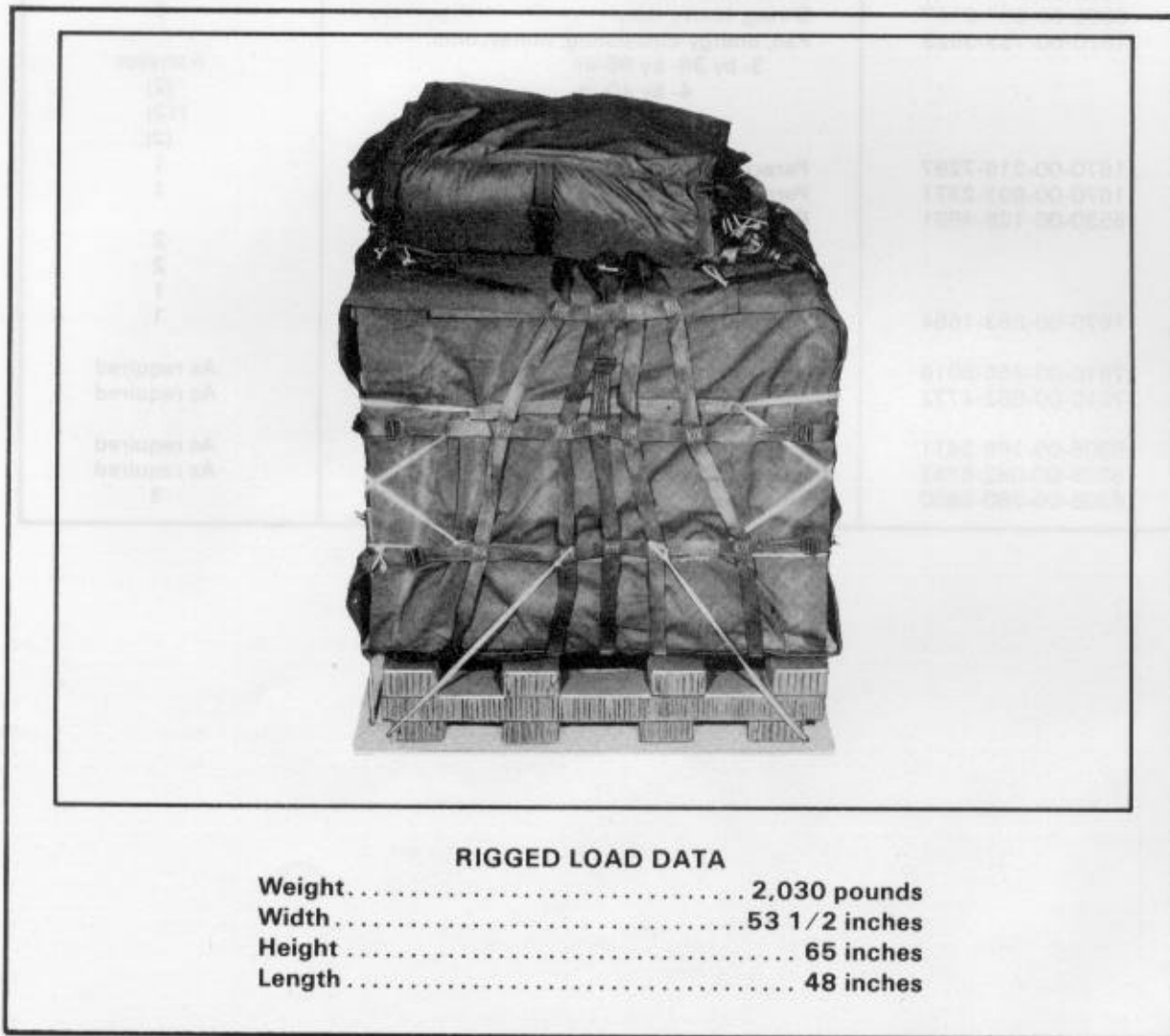
Figure 3-9. Milk-dispensing containers rigged in A-22 cargo bag for low-velocity airdrop.
